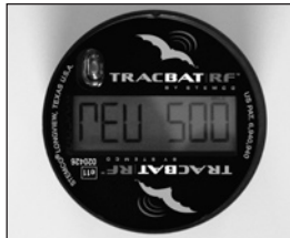
REV Mode shows RPM or RPK.
